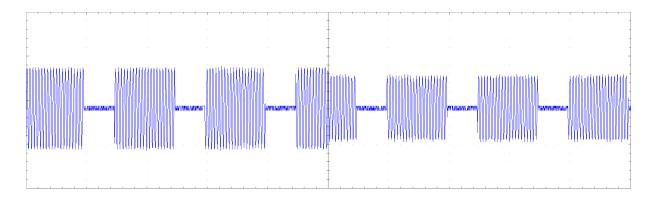
*Figure 3: Changing power setting with blanking disabled while pulse modulation is active (1 ms pulse, 0.5 ms space).*
