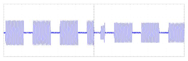
*Figure 2: Changing power setting with blanking enabled (default mode) while pulse modulation is active (1 ms pulse, 0.5 ms space).*
